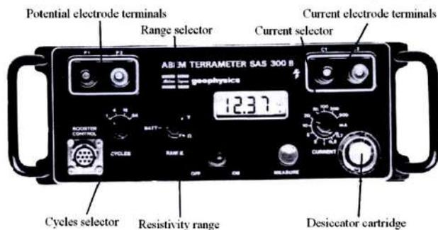
**Figure 2: ABEM TERRAMETER SAS 300B resistivity meter.**
