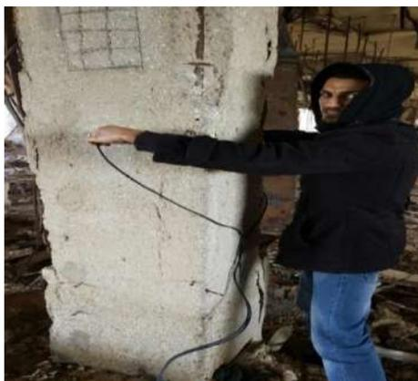
**Figure 9: Usage of ultrasonic pulse velocity test.**
