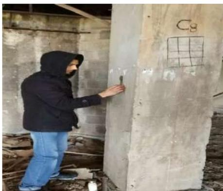
**Figure 8: Preparation of surface of column to UPV test.**
