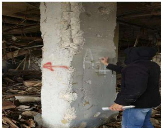
**Figure 4: Preparation of surface of column test I.**
