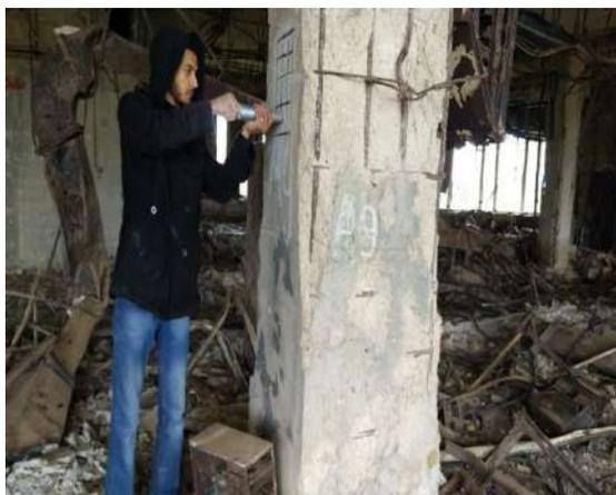
**Figure 6: Usage of rebound hammer test.**
